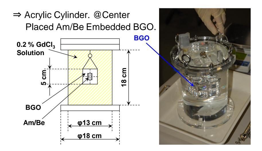
... This Apparatus Deployed @Detector Center in SK.
