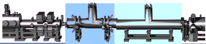
**DPS:** differential pumping of T<sub>3</sub> using TMPs (2000 l/s) • 6.2 m long • 5 solenoids • with B = 5.6 T  $\rightarrow$  T<sub>2</sub> reduction by 10<sup>7</sup>
