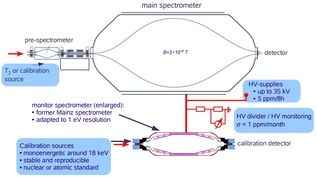
**error budget:**  $\Delta m_v^2 \le 0.007 \text{ eV}^2 \implies \sigma < 60 \text{ meV} \implies 3 \text{ ppm long term stability}$
