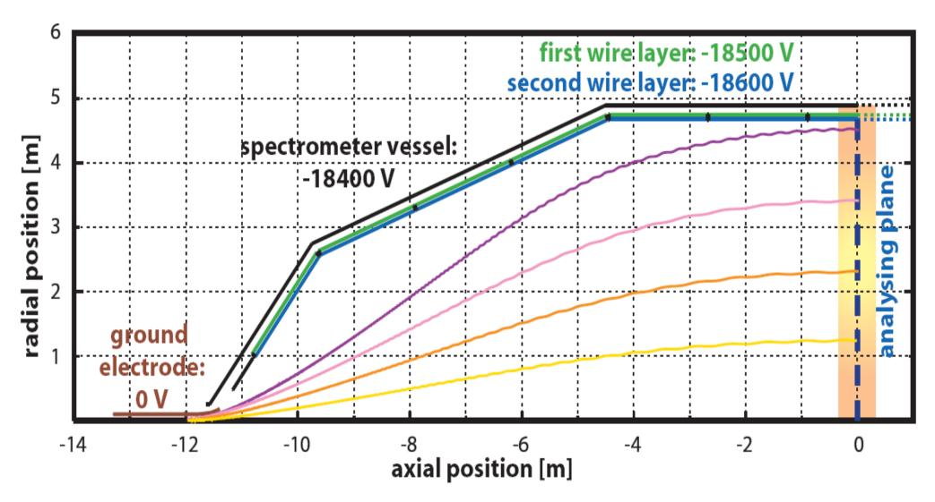
overview: electrode system of the main spectrometer
