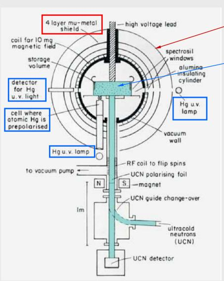
4 layers of passive (μ-metal) shield
